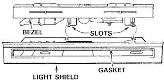
To reinstall the light shield, first position the gasket at the top so that the flap is toward the front. Then, position the lower edges of the light shield firmly into the slots in the mounting supports. Lift the top edge of the light shield and engage it over the top of the bezel.
