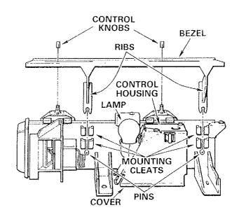
To reinstall the bezel, first position the knob shafts to the extreme left positions. Then, engage the ribs into the mounting cleats and press each rib firmly to seat the slots on the pins.
